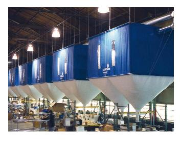
Storopack offers custom integration systems that conveniently store RENATURE® and deliver it to individual packing stations. Bulk trucks load the loose fill product directly into a delivery system quickly and efficiently, keeping your production lines working at full capacity.
